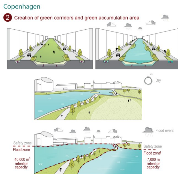
Figure 2. COPENHAGEN: The Copenhagenize Current - Stormwater Management and Cycle Tracks . Here the second strategy: creation of green corridors and green accumulation area
